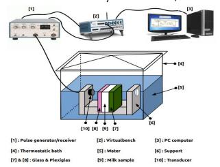
Figure 1. Ultrasonic experimental characterization system
