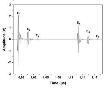
Figure 2. Time domain backscattered signals from milk sample.
