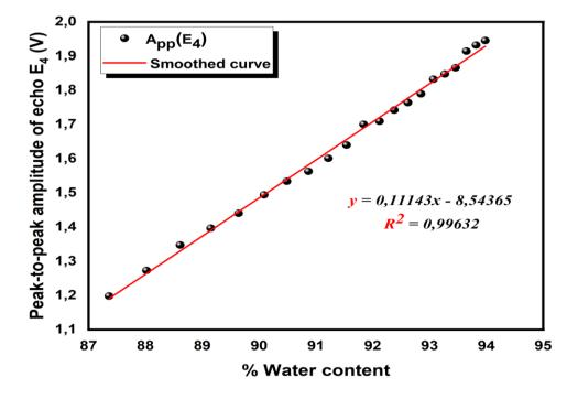
Figure 4. Peak-to-peak amplitude of echo E4 for adulterated milk samples versus different amounts of adulterant
