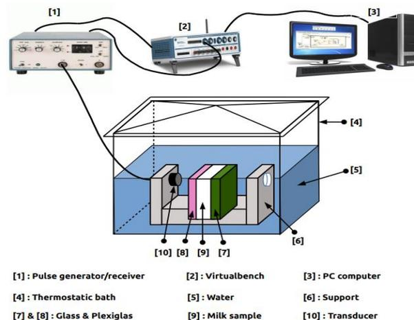
Figure 1. Ultrasonic experimental characterization system
